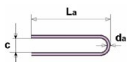
Angle Lift Reinforcement
