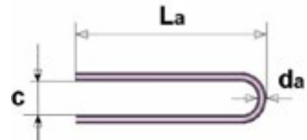
Angle Lift Reinforcement
